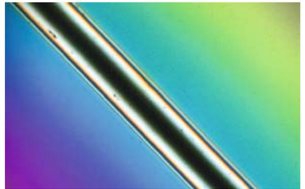
Nylon fiber, polarization, Berek compensator 0 to 5  $\lambda$
